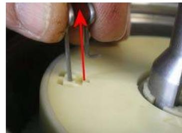
10) Reassemble hose, gasket and elastic ring.
